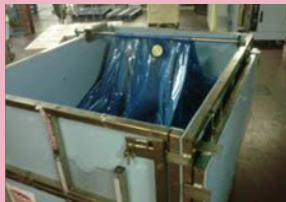
Pallecon with plastic liner bag
